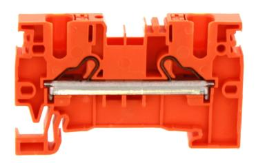
Feed-through terminal, Push-in connection, Mounting type: Mounting rail TS 35/7.5, Rated cross-section: 4 mm², Width: 6.1 mm, Colour: Orange
