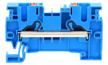
Feed-through terminal, Push-in connection, Mounting type: Mounting rail TS 35/7.5, Rated cross-section: 4 mm<sup>2</sup>, Width: 6.1 mm, Colour: Blue
