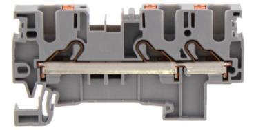
Feed-through terminal, Push-in connection, Mounting type: Mounting rail TS 35/7.5, Rated cross-section: 4 mm<sup>2</sup>, Width: 6.1 mm, Colour: Grey
