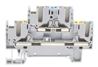
Double-level terminal, Push-in connection, Mounting type: Mounting rail TS 35/7.5, Rated cross-section: 2.5 mm², Width: 5.1 mm, Colour: Grey
