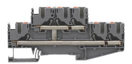
Double-level terminal, Push-in connection, Mounting type: Mounting rail TS 35/7.5, Rated cross-section: 4 mm², Width: 6.1 mm, Colour: Grey
