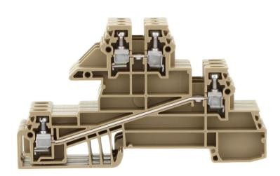
Three-wire installation terminal, Screw connection, Mounting type: Mounting rail TS 35/7.5, Rated cross-section: 2.5 mm², Width: 18 mm, Colour: Beige
