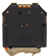
Feed-through terminal, Screw connection, Mounting type: Mounting rail TS 35/7.5 and TS 32, Rated cross-section: 150 mm<sup>2</sup>, Width: 31 mm, Colour: Black-yellow
