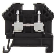
Feed-through terminal, Screw connection, Mounting type: Mounting rail TS 35/7.5, Rated cross-section: 4 mm<sup>2</sup>, Width: 6 mm, Colour: Black
