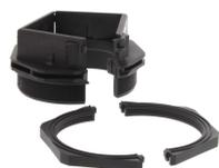
Split cable gland including counter nut, Thread type: metric, Material: PA 6.6, Protection: IP 66, Colour: Black
