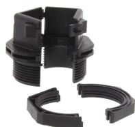
Split cable gland including counter nut, Thread type: metric, Material: PA 6.6, Protection: IP 66, Colour: Black
