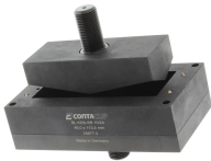
Sheet metal punch for rectangular openings, Dimensions opening: 46 x 46 mm, Maximum wall thickness: 2.0 mm for stainless steel sheet, Material: steel
