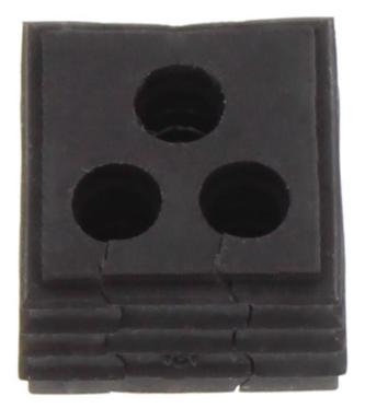
Seal, Mounting type: Plug in, Length x width: 20.3 mm, Max. cable diameter: 6.5 mm, IP 66, Colour: Black
