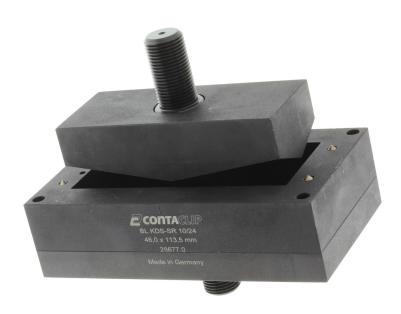
Sheet metal puncher for rectangular openings, Dimensions opening:  $46 \times 24 \text{ mm}$ , Maximum wall thickness: 2.0 mm for stainless steel sheet, Material: steel
