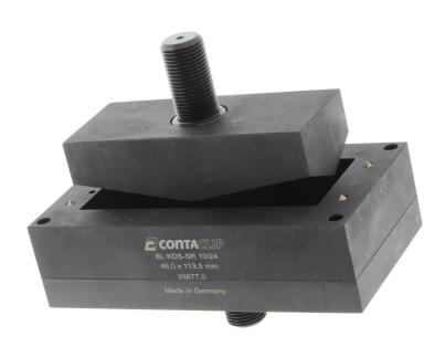
Sheet metal puncher for rectangular openings, Dimensions opening: 112 x 36 mm, Maximum wall thickness: 2.0 mm for S 235 sheet, Material: steel
