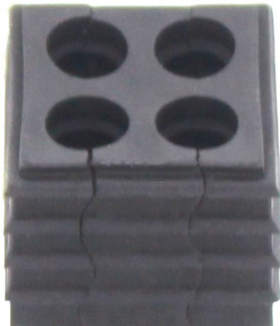
Seal, Mounting type: Plug in, Length x width: 20.3 mm, Max. cable diameter: 6.1 mm, IP 66, Colour: Black
