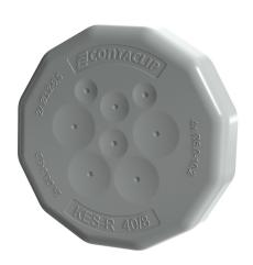
Round cable entry M40 with membrane for non-assembled cables, Mounting type: Snap-in and Screw, Length: 51 mm, Width: 51 mm, IP66, Colour: Grey
