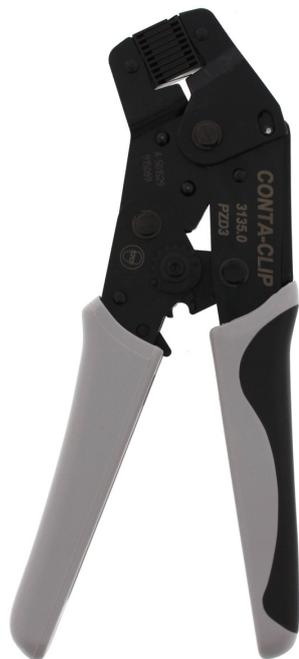
Crimping tool for crimping wire-end ferrules with and without plastic collars. Cross-section range: 0.5-6 mm<sup>2</sup> (AWG 2-10). Easy to use, Auto-lock for proper and complete crimping, Wires fed in from the front, Self-opening with built-in spring.
