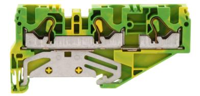
PE installation terminal, Push-in connection, Mounting type: Mounting rail TS 35/7.5, Rated cross-section: 10 mm<sup>2</sup>, Width: 8.1 mm, Colour: Green-yellow
