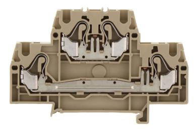
Double-level terminal with housing pegs, block variant, Push-in connection, Mounting type: Mounting rail TS 35/7.5, Rated cross-section: 2.5 mm<sup>2</sup>, Width: 5.1 mm, Colour: Beige
