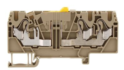
Disconnect-blade terminal, Push-in connection, Mounting type: Mounting rail TS 35/7.5, Rated cross-section: 2.5 mm², Width: 5.1 mm, Colour: Beige
