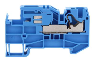
Neutral-disconnect terminal, Push-in connection, Mounting type: Mounting rail TS 35/7.5, Rated cross-section: 10 mm², Width: 8.1 mm, Colour: Blue
