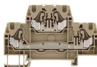
Double-level terminal, Push-in connection, Mounting type: Mounting rail TS 35/7.5, Rated cross-section: 2.5 mm<sup>2</sup>, Width: 5.1 mm, Colour: Beige
