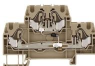
Double-level terminal with electronic components, Push-in connection, Mounting type: Mounting rail TS 35/7.5, Rated cross-section: 2.5 mm<sup>2</sup>, Width: 5.1 mm, Colour: Beige
