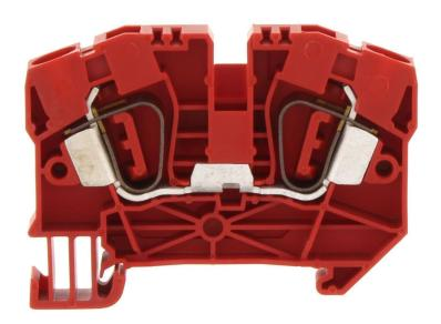
Feed-through terminal, Tension-spring connection, Mounting type: Mounting rail TS 35/7.5, Rated cross-section: 6 mm², Width: 8.1 mm, Colour: Red
