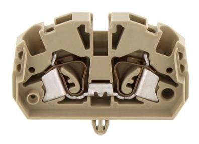
Feed-through terminal for direct mount, Tension-spring connection, Mounting type: Mounting surface, Rated cross-section: 2.5 mm², Width: 5.1 mm, Colour: Beige
