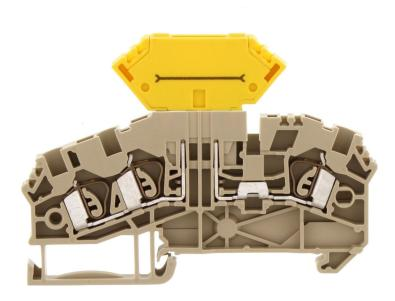
Disconnect terminal, Tension-spring connection, Mounting type: Mounting rail TS 35/7.5, Rated cross-section: 2.5 mm², Width: 5.1 mm, Colour: Beige
