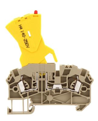
Fuse-disconnect terminal, Tension-spring connection, Mounting type: Mounting rail TS 35/7.5, Rated cross-section: 2.5 mm², Width: 5.1 mm, Colour: Beige
