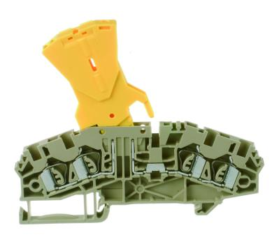
Fuse-disconnect terminal, Tension-spring connection, Mounting type: Mounting rail TS 35/7.5, Rated cross-section: 2.5 mm², Width: 5.1 mm, Colour: Beige
