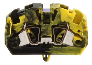
Feed-through terminal for direct mount, Tension-spring connection, Mounting type: Mounting surface, Rated cross-section: 2.5 mm<sup>2</sup>, Width: 5.1 mm, Colour: Black-yellow
