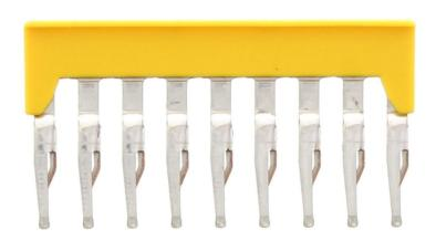
Insulated cross-connector, No. of poles: 9, Mounting type: Plug in, Width: 44.8 mm, Rated cross-section: 2.5 mm<sup>2</sup>, Colour: Yellow
