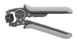
Crimping tool for crimping ferrules with and without plastic collars. Cross section range: 0.08-16 mm<sup>2</sup> (AWG 28-5). Easy to use, forced lock for correct, complete crimping, conductor entry can be rotated in 45° steps, self-opening thanks to built-in spring.
