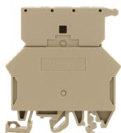
Fuse-disconnect terminal, Screw connection, Mounting type:Mounting rail TS 35/7.5 and TS 32, Rated cross-section: 10 mm<sup>2</sup>, Width: 10 mm, Colour: Beige
