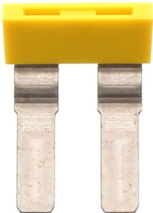
External insulated cross-connector, No. of poles: 2, Mounting type: Plug in, Width: 18.1 mm, Rated current: 57 A; Colour: Yellow
