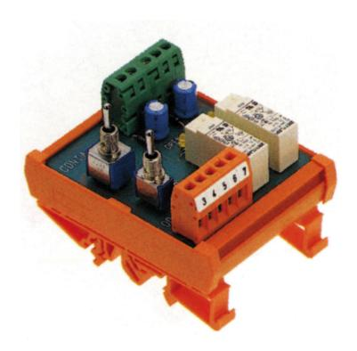
Digital switching module with manual-off-automatic switching, additional switch for open/stop/close and watchdog, Screw connection, Mounting type: Mounting rail TS 35, 1 channel, Voltage: 24 VAC/DC
