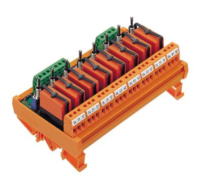
Multiple relay module with manual actuation, Screw connection, With 4 miniature relays, 1 CO contact each, Plugged in, With illuminated display, Separated channels, Input voltage: 24 VAC
