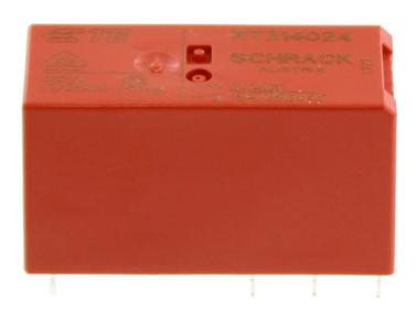
Plug-in miniature power relay, Encapsulated design with power contact, 1 CO contact, Input voltage: 24 VDC
