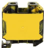
Feed-through terminal, Screw connection, Mounting type: Mounting rail TS 35/7.5, Rated cross-section: 35 mm<sup>2</sup>, Width: 16.1 mm, Colour: Black-yellow
