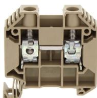
Feed-through terminal, Screw connection, Mounting type: Mounting rail TS 35/7.5, Rated cross-section: 16 mm<sup>2</sup>, Width: 12.1 mm, Colour: Beige
