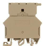
Fused terminal with disconnect plug, Screw connection, Mounting type: Mounting rail TS 35/7.5 and TS 32, Rated cross-section: 10 mm<sup>2</sup>, Width: 10 mm, Colour: Beige
