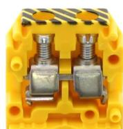
Feed-through terminal for direct mount, Screw connection, Mounting type: Mounting surface, Rated cross-section: 4 mm<sup>2</sup>, Width: 6 mm, Colour: Black-yellow
