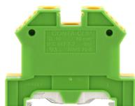
Protective earth terminal, Screw connection, Mounting type: Mounting rail TS 35/7.5, Rated cross-section: 10 mm<sup>2</sup>, Width: 10 mm, Colour: Green-yellow
