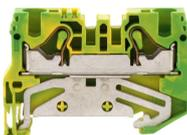
PE installation terminal, Push-in connection, Mounting type: Mounting rail TS 35/7.5, Rated cross-section: 10 mm<sup>2</sup>, Width: 8.1 mm, Colour: Green-yellow
