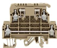
Disconnect terminal, Screw connection, Mounting type: Mounting rail TS 35/7.5 and TS 32, Rated cross-section: 4 mm<sup>2</sup>, Width: 8 mm, Colour: Beige
