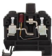
Fused terminal, Screw connection, Mounting type: Mounting rail TS 35/7.5, Rated cross-section: 10 mm<sup>2</sup>, Width: 12.2 mm, Colour: Black
