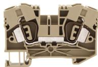
Feed-through terminal, Tension-spring connection, Mounting type: Mounting rail TS 35/7.5, Rated cross-section: 10 mm<sup>2</sup>, Width: 10.1 mm, Colour: Beige
