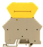
Disconnect terminal, Screw connection, Mounting type: Mounting rail TS 15/5.5, Rated cross-section: 2.5 mm<sup>2</sup>, Width: 6 mm, Colour: Beige
