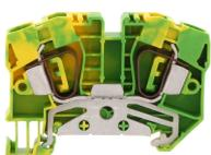
Ex protective-earth terminal ATEX-certified Tension-spring connection, Mounting type: Mounting rail TS 35/7.5, Rated cross-section: 6 mm<sup>2</sup>, Width: 8.1 mm, Colour: Green-yellow
