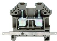
Feed-through terminal, Screw connection, Mounting type: Mounting rail TS 35/7.5, Rated cross-section: 10 mm<sup>2</sup>, Width: 8 mm, Colour: Beige
