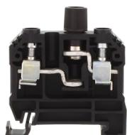
Fused terminal with screw cap for indicator fuses 5x25 mm, Screw connection, Mounting type: Mounting rail TS 35/7.5, Rated cross-section: 10 mm<sup>2</sup>, Width: 12.2 mm, Colour: Black
