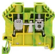
EX-Protective earth terminal, Screw connection, Mounting type: Mounting rail TS 35/7.5, Rated cross-section: 16 mm<sup>2</sup>, Width: 10 mm, Colour: Green-yellow
