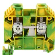
Protective earth terminal, Screw connection, Mounting type: Mounting rail TS 35/7.5, Rated cross-section: 16 mm<sup>2</sup>, Width: 12.1 mm, Colour: Green-yellow
