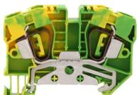
Protective earth terminal, Tension-spring connection, Mounting type: Mounting rail TS 35/7.5, Rated cross-section: 6 mm<sup>2</sup>, Width: 8.1 mm, Colour: Green-yellow
