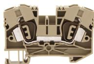
Ex feed-through terminal ATEX-certified, Tension-spring connection, Mounting type: Mounting rail TS 35/7.5, Rated cross-section: 10 mm<sup>2</sup>, Width: 10.1 mm, Colour: Beige
