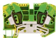
Ex protective-earth terminal ATEX-certified Tension-spring connection, Mounting type: Mounting rail TS 35/7.5, Rated cross-section: 10 mm<sup>2</sup>, Width: 10.1 mm, Colour: Green-yellow
