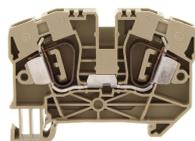
Ex feed-through terminal ATEX-certified, Tension-spring connection, Mounting type: Mounting rail TS 35/7.5, Rated cross-section: 6 mm<sup>2</sup>, Width: 8.1 mm, Colour: Beige
