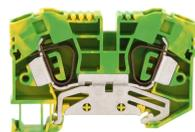
Protective earth terminal, Tension-spring connection, Mounting type: Mounting rail TS 35/7.5, Rated cross-section: 10 mm<sup>2</sup>, Width: 10.1 mm, Colour: Green-yellow
