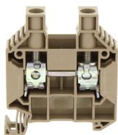
Feed-through terminal, Screw connection, Mounting type: Mounting rail TS 35/7.5, Rated cross-section: 16 mm<sup>2</sup>, Width: 12.1 mm, Colour: Beige
