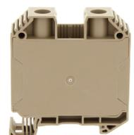
Feed-through terminal, Screw connection, Mounting type: Mounting rail TS 35/7.5, Rated cross-section: 35 mm<sup>2</sup>, Width: 16.1 mm, Colour: Beige
